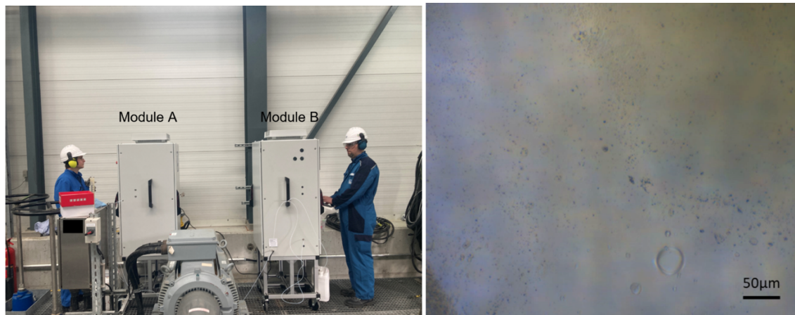
Figure 18: Modules A & B connected and measuring OMV WTP process stream (left); Particles, air bubbles and oil droplets on the optical window (right).
