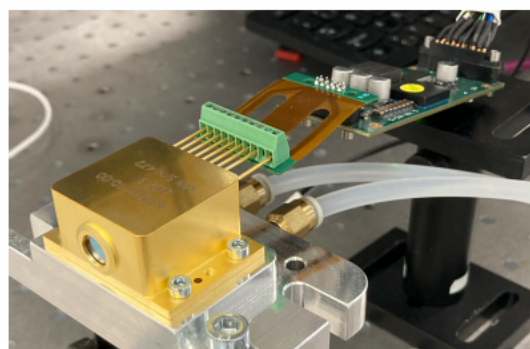
Figure 8. Fully packaged PIC in a HHL module connected to a S2-M driver.
